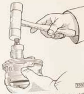
Fig. 26. Removing the pressure plate, pump ring and thrust plate assembly.
