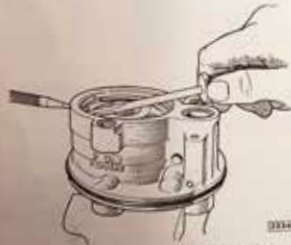
Fig. 27. Removing the end plate retaining ring.
